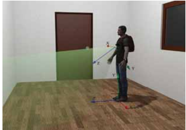
Fig. 1 Wearable camera position: the RGB-D sensor is chest mounted and it looks downwards 45°; the laptop where all the computation is carried on is on the backpack. The image shows the field of view of the sensor (green) and the axis of the scene ( X'-Y'-Z' ) and the sensor ( X-Y-Z ).
